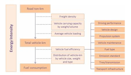
Fig. 24. Direct and indirect factors that affect the energy consumption in the road transport sector Source: Adapted from (Piecyk & Mckinnon 2009)
